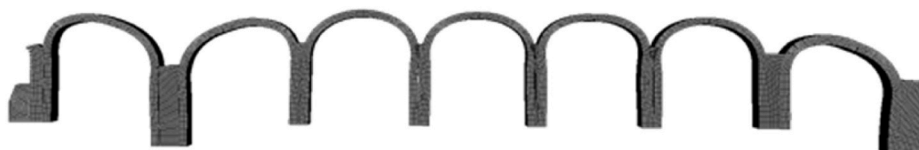
Fig. 25. Deformation shape of the structure after a 100 kN horizontal point load has been applied on the further left hand-side abutment together with a 100 mm vertical displacement on the 100 mm vertical displacement of the second and eight support.
